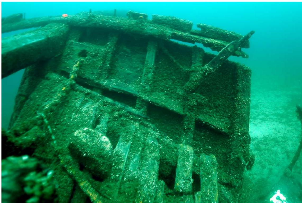
Figure 27. Starboard side bow with outer hull planks, frames, breasthook, and dislodged deck beam and planking. Photo by Tamara Thomsen.
