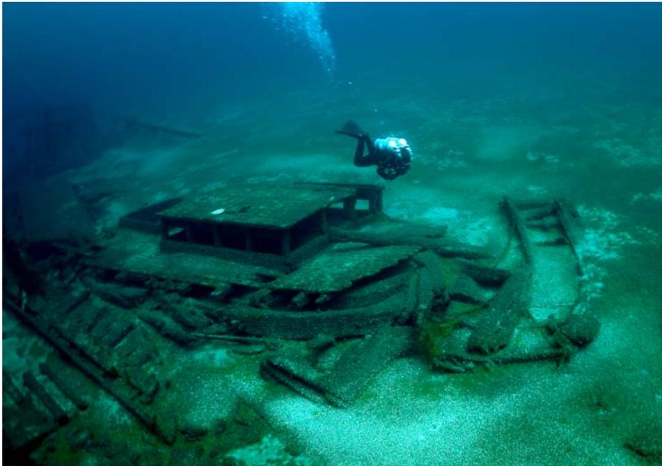
Figure 18. *Ocean Wave*'s transom, rudder, aft deck, and cabin. Photo by Tamara Thomsen.
