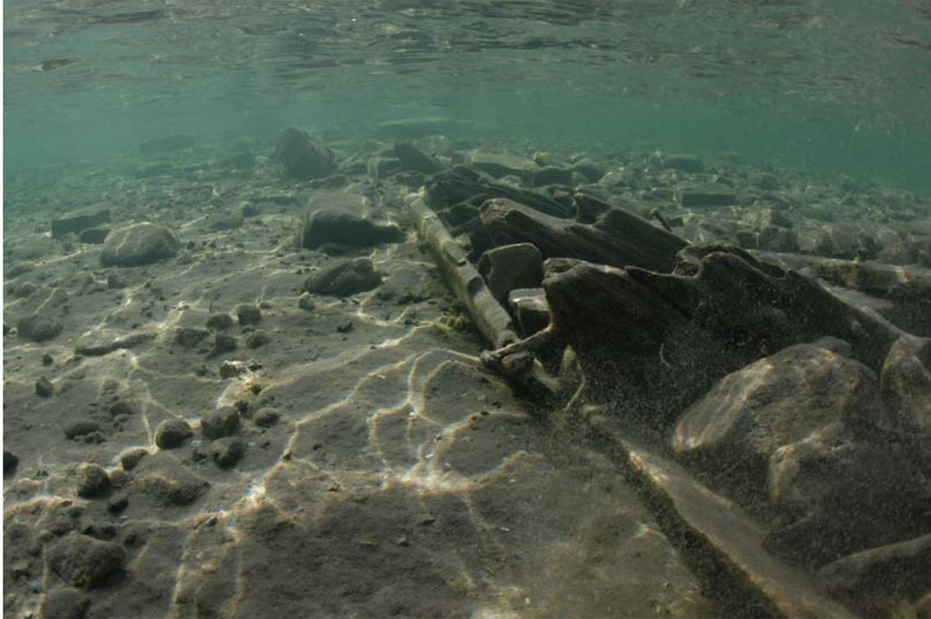
Figure 10. Frames and outer hull planking at the turn of the bilge, port quarter. Photo by Tamara Thomsen.
