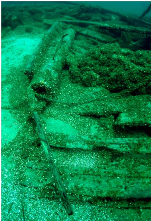
Figure 30. Bilge pump aft of chain locker. Photo by Tamara Thomsen.
