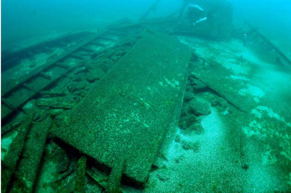
Figure 19. Centerboard trunk with centerboard protruding from bottom. Photo by Tamara Thomsen.
