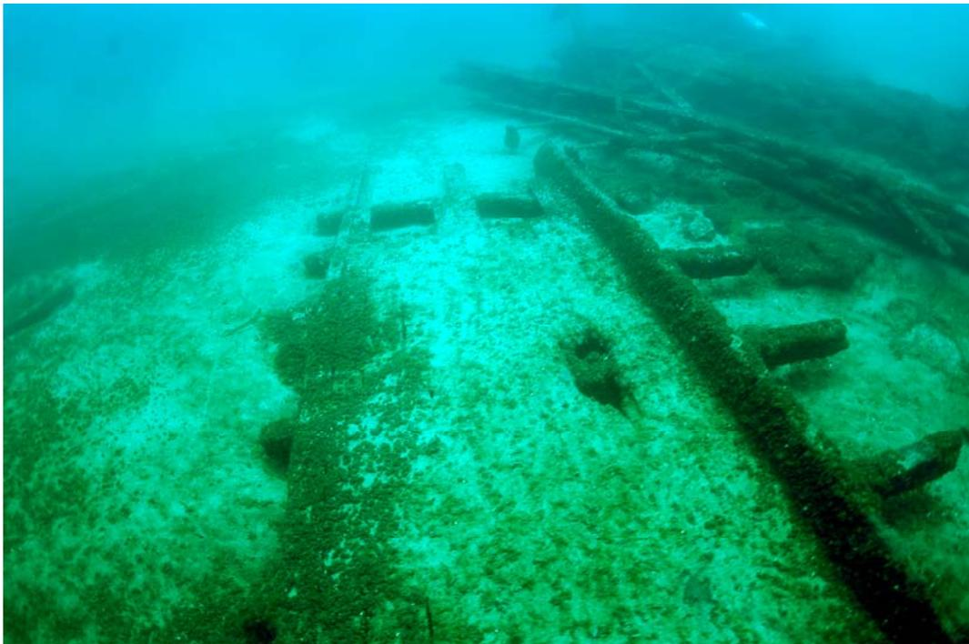
Figure 24. Forward hatch combing and deck, facing north. Note three deck beams protruding beneath combing. Photo by Tamara Thomsen.
